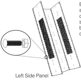
Bolt the tamper-proof screw on the inside of the locker. Only the screw heads should be visible from the outside of the locker.
